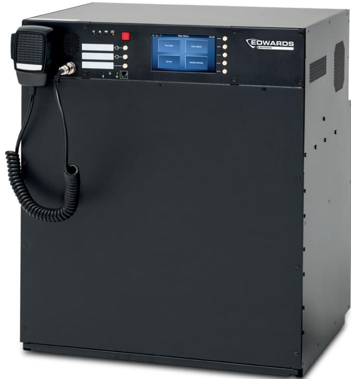
EST VES is scalable Public Address & Voice Alarm unit suitable for multi-purpose architectures. Devices from EST VES series are voice alarm compact control units containing all components within one compact housing, which meet all the requirements of EN 54-16 and EN 54-4 (certificate of constancy of performance 1438-CPR-XXXX).
